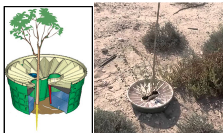
Figure 4. An illustration of Waterboxx (left) and a tree planted using a Waterboxx (right). Picture of a product from Spain. https://www.youtube.com/watch?v=jvc1Wm9KKro
